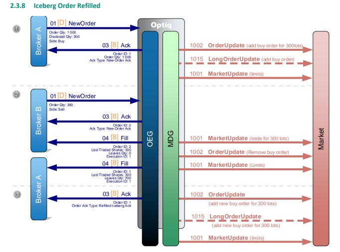
Image: Broker A sends a private NewOrder (01) (FIX D) message to enter a new Buy Iceberg order with a quantity of 1,000 and a Disclosed Quantity of 300.
