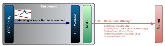
When the underlying price breaches the deactivation barrier of the warrant instrument, the warrant is automatically Knock-Out. A public **MarketStatusChange** (1005) message is sent to the market to communicate the suspension of the instrument (Status Reason 'Knock-Out by Exchange'). The order entry is set to Cancel Only and LP quotes (if any) are automatically cancelled.
