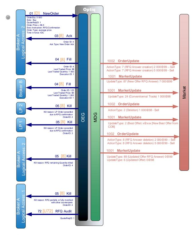
The broker A (RFQ issuer) from Logical Access 2 confirms the RFQ with a **NewOrder** (01) (FIX D) message with a quantity of 5 000 and a price of 98.5.
