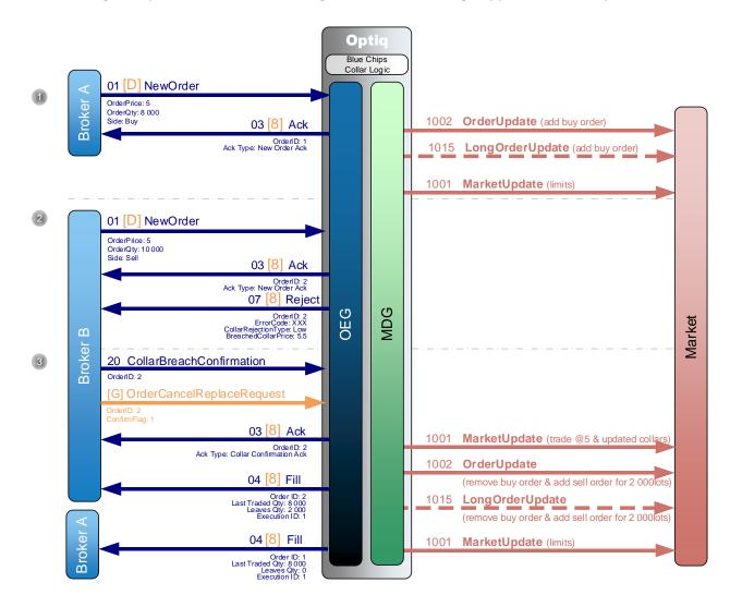
Broker A sends a private NewOrder (01) (FIX D) message to enter a new Buy order with a quantity of 8,000 and a price=5, which is lower than the low collar. OEG sends back a private **Ack** (03) (FIX 8) message to confirm the successful receipt and technical processing of the order.
