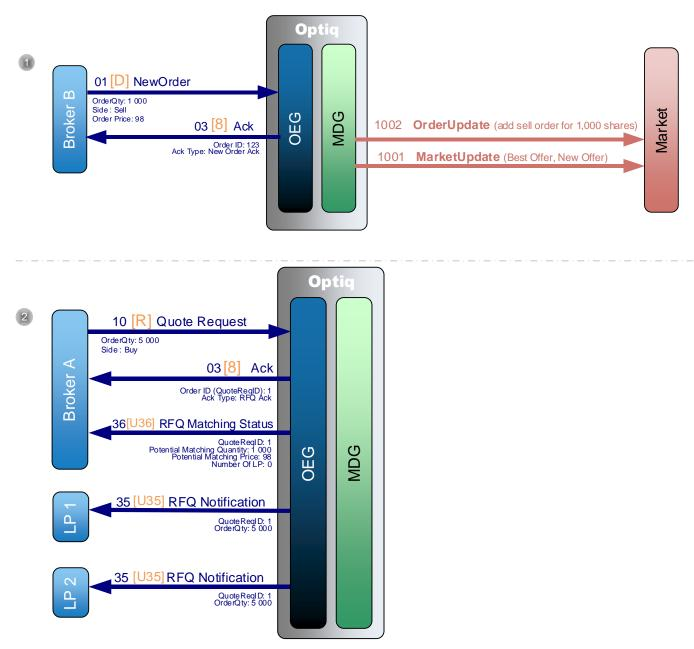
① A Broker sends a private **NewOrder** (01) (FIX D) message to enter a new Buy order with a quantity of 1,000. OEG sends back a private **Ack** (03) (FIX 8) message to confirm the successful receipt and technical processing of the order.
