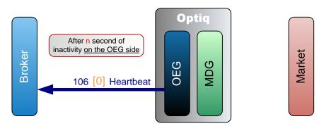
After *n* second(s) of inactivity on its side (ie. when the OEG has not sent any message since *n* second(s)) the OEG sends a **Heartbeat** (106) (FIX 0) message to the broker. The broker does not have to respond anything; it is only a notification from the OEG.
