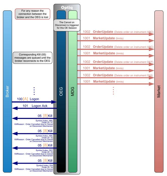
The diagram represents a generic case of loss of connection (physical) between a client and a partition.
