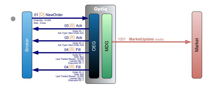
① A Broker sends a private **NewOrder** (01) (FIX D) message to enter a new order with a quantity of 10,000 and a Cross side.
