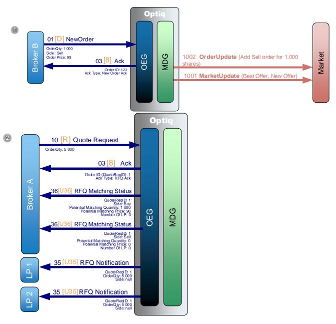
In Broker B sends a private NewOrder (01) (FIX D) message to enter a new Sell order with a quantity of 1,000. OEG sends back a private Ack (03) (FIX 8) message to confirm the successful receipt and technical processing of the order.
