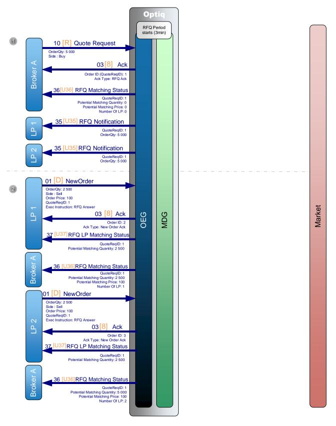
① A Broker sends a private QuoteRequest (10) (FIX R) message to broadcast a new RFQ order with a quantity of 5 000. OEG sends back a private Ack (03) (FIX 8) message to confirm the successful receipt and technical processing of the RFQ. This Ack message is an "RFQ Ack", as a consequence the Order ID will contain the QuoteReqID.
