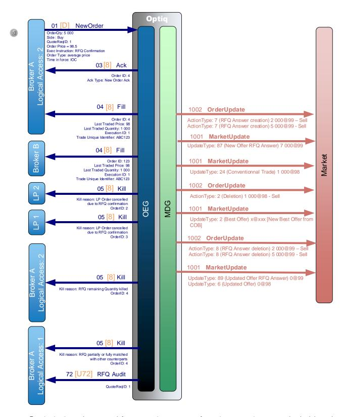
⑤ The broker A (RFQ issuer) from Logical Access 2 confirms the RFQ with a **NewOrder** (01) (FIX D) message with a quantity of 5 000 and a price of 98.5.
