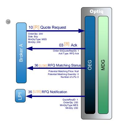
2) A Broker sends a private **Quote Request** (10) (FIX R) message to broadcast a new RFQ order with a quantity of 200 with a Minimum Executable Size (MES) of 200. OEG sends back a private **Ack** (03) (FIX 8) message to confirm the successful receipt and technical processing of the RFQ. This Ack message is an "RFQ Ack", as a consequence the *Order ID* will contain the QuoteReqID.
