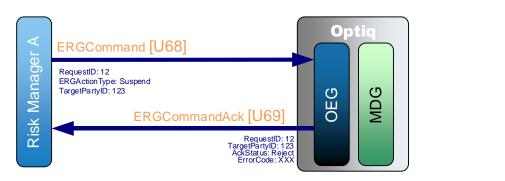
Risk Manager A sends a private **ERGCommand** (U68) message to suspend a trader or an algorithm using a Short Code, without providing the *Firm ID*.
