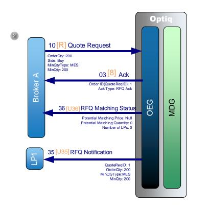
2) A Broker sends a private **Quote Request** (10) (FIX R) message to broadcast a new RFQ order with a quantity of 200 with a Minimum Executable Size (MES) of 200. OEG sends back a private **Ack** (03) (FIX 8) message to confirm the successful receipt and technical processing of the RFQ. This Ack message is an "RFQ Ack", as a consequence the *Order ID* will contain the QuoteReqID.
