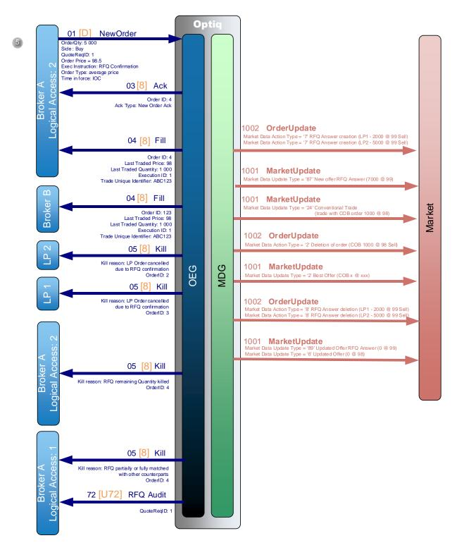
5) The broker A (RFQ issuer) from Logical Access 2 confirms the RFQ with a **NewOrder** (01) (FIX D) message with a quantity of 5 000 and a price of 98.5.
