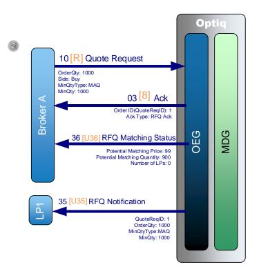
2) A Broker sends a private **Quote Request** (10) (FIX R) message to broadcast a new RFQ order with a quantity of 1,000 with a Minimum Acceptable Quantity (MAQ) of 1,000. OEG sends back a private **Ack** (03) (FIX 8) message to confirm the successful receipt and technical processing of the RFQ. This Ack message is an "RFQ Ack", as a consequence the *Order ID* will contain the QuoteReqID.
