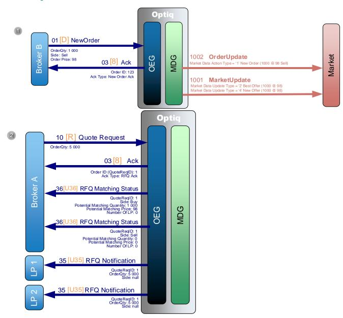
1) Broker B sends a private **NewOrder** (01) (FIX D) message to enter a new Sell order with a quantity of 1,000. OEG sends back a private **Ack** (03) (FIX 8) message to confirm the successful receipt and technical processing of the order.
