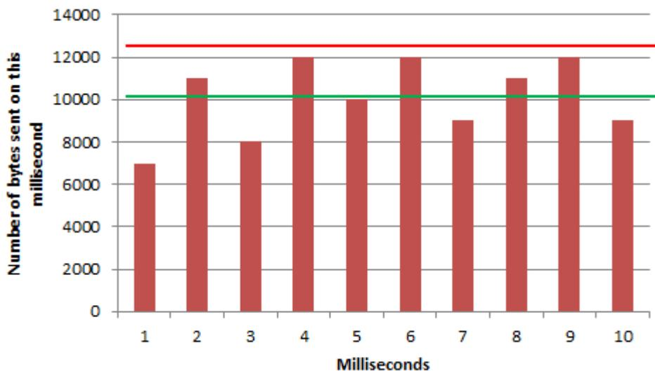
We can see that nothing uses more than the bandwidth acceptance (red line) and the average use of the bandwidth (green line) is lower (10 100 bytes per millisecond).
