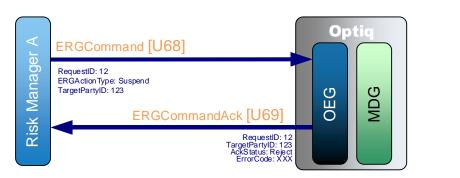
Risk Manager A sends a private **ERGCommand** (U68) message to suspend a trader or an algorithm using a short code, without providing the Firm ID.
