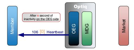
After n second(s) of inactivity on Optiq OEG session side (i.e. when the OEG has not sent any message since n second(s)) the OEG sends a **Heartbeat** (106) (FIX 0) message to the member to signify that the connection is still alive from Optiq perspective. The member does not have to respond; it is only a notification from the OEG.
