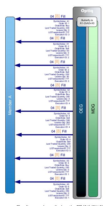
The diagram above displays the **Fill** (04) (FIX 8) message sent to Member A for the crossed quantity on all the submitted legs, as well as the matches against Member B on the A1 and A2. The associated public messages are described in the diagram above.
