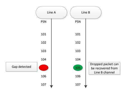
Using this method, a lost packet can be recovered from the second line. In case of packet loss on both lines, then the snapshot mechanism should be used.
