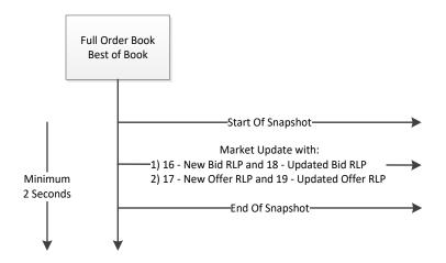
Both "Start Of Snapshot" and "End Of Snapshot" messages contain the last "Market Data Sequence Number" of the last real-time message taken into account by the snapshot (see <u>Sequence Numbers</u> and <u>Snapshot Sequence behaviour</u> for explanations on the "Market Data Sequence Number"). This last MDSN has been sent on each channel speed.
