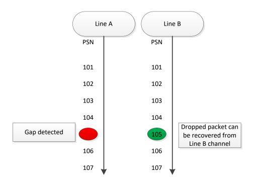
Using this method, a lost packet can be recovered from the second line. In case of packet loss on both lines, then the snapshot mechanism should be used.
