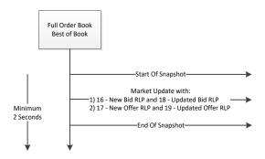
Both "Start Of Snapshot" and "End Of Snapshot" messages contain the last "Market Data Sequence Number" of the last real-time message taken into account by the snapshot (see <u>Sequence Numbers</u> and <u>Snapshot Sequence behaviour</u> for explanations on the "Market Data Sequence Number"). This last MDSN has been sent on each channel speed.
