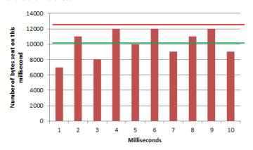
We can see that nothing uses more than the bandwidth acceptance (red line) and the average use of the bandwidth (green line) is lower (10 100 bytes per millisecond).
