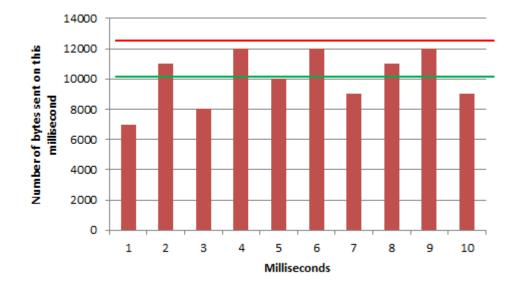
We can see that nothing uses more than the bandwidth acceptance (red line) and the average use of the bandwidth (green line) is lower (10 100 bytes per millisecond).
