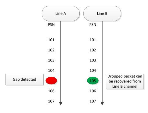
Using this method, a lost packet can be recovered from the second line. In case of packet loss on both lines, then the snapshot mechanism should be used.
