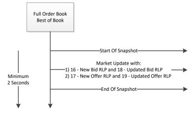
Both **Start Of Snapshot** (2101) and **End Of Snapshot** (2102) messages contain the last *Market Data Sequence Number* (MDSN) of the last real-time message taken into account by the snapshot (see <u>Sequence Numbers</u> and <u>Snapshot Sequence behaviour</u> for explanations on the MDSN). This last MDSN has been sent on each channel speed.
