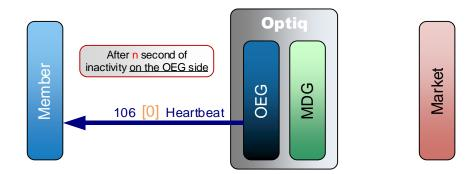
After n second(s) of inactivity on Optiq OEG session side (i.e. when the OEG has not sent any message since n second(s)) the OEG sends a **Heartbeat** (106) (FIX 0) message to the member to signify that the connection is still alive from Optiq perspective. The member does not have to respond; it is only a notification from the OEG.
