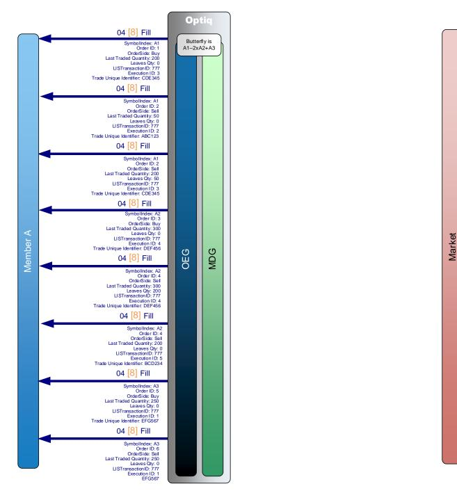
The diagram above displays the **Fill** (04) (FIX 8) message sent to Member A for the crossed quantity on all the submitted legs, as well as the matches against Member B on the A1 and A2. The associated public messages are described in the diagram above.
