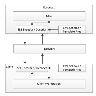
SBE offers the possibility to have backward and forward compatibility. It means that clients are not required to be on the last version of Schema Version (message structure version) to be able to read the message. This is only possible if changes between versions occurred at the end of:
